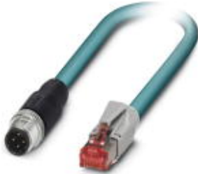
Assembled Ethernet cable, CAT5e, shielded, 2-pair, AWG 26, stranded (7-wire), RAL 5021 (aqua blue), M12 plug to RJ45 plug/IP20, line, length 3 m
