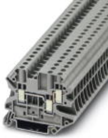
Feed-through terminal block, Connection method: Screw connection, Cross section: 0.14 mm 2 - 6 mm 2 , AWG: 26 - 10, Width: 6.2 mm, Color: gray, Mounting type: NS 35/7,5, NS 35/15
