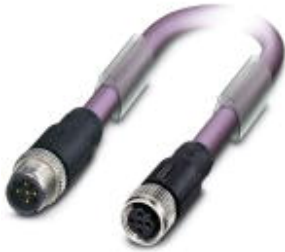
Bus system cable, PROFIBUS, PROFIBUS, 2-position, PUR halogen-free, Violet, RAL 4001, shielded, Plug straight M12, B-coded, on Socket straight M12, B-coded, Cable length: 1 m
