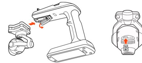
**STEP 1)** Remove the protective cover for the contactor as illustrated.
