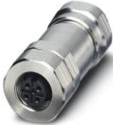
Connector, 5-position, shielded, Socket straight M12, A-coded, Screw connection, Knurl material: Stainless steel, Cable gland M16, External cable diameter 5.5 mm ... 8.6 mm
