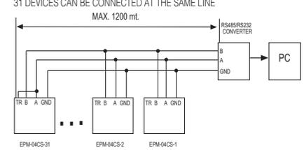
MAX. 247 DEVICES CAN BE CONNECTED AT SAME LINE BY USING REPEATER.
